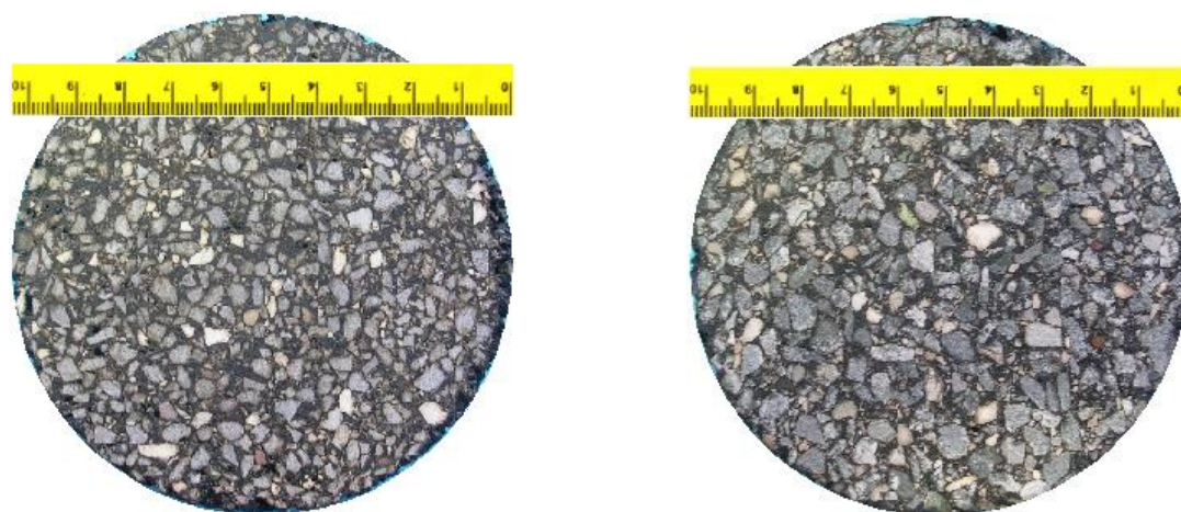
Gap Graded Asphalt Mixture by the Dry Process (GGD)
