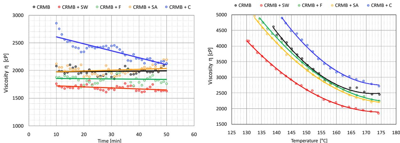
Figure 1: Isotherm viscosity curves at T=175°C and the viscosity curves versus temperature.
