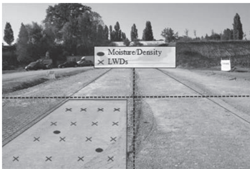
Figure 10. Positioning of the test points for every layer.
