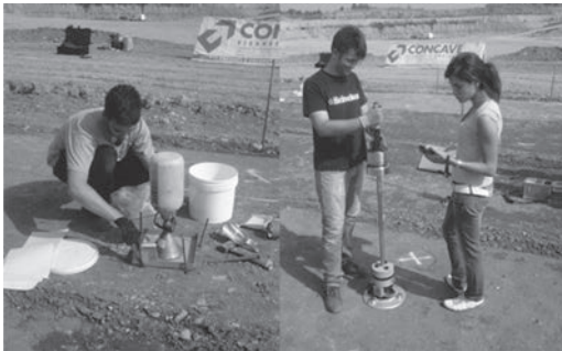
Figure 9. Density tests (a) and bearing capacity tests using a LWD (b).
