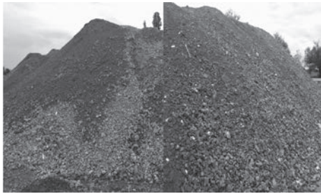
Figure 1. C&D from the demolition of selected concrete masonry (left) and non-selective masonry from buildings and other constructions (right).
