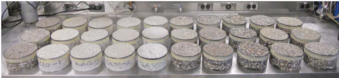
Fig. 2. Core samples selected for sound absorption testing.
