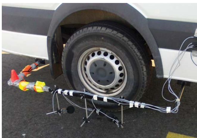
Fig. 4. Layout of the CPX and OBSI noise testing setup.
