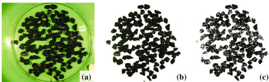
Fig. 2 Image filtering process. a Original image; b Non-classified image; c Classified image
