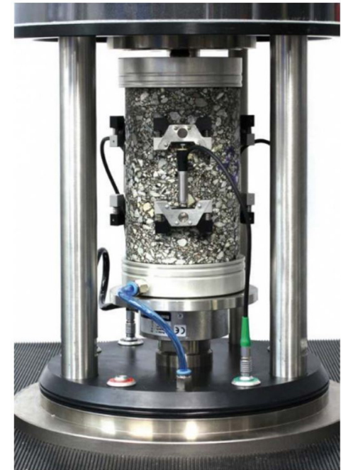
AMPT configuration for the Dynamic Modulus test
